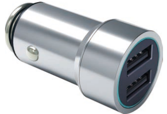
Model: CP31B Input: DC 12-24V Output: USB*2 5V 2.4A each port, Total 5V/3.4A Chromed Copper, Blue LED light in circle Dimension: 53.4*25.4*20.3mm Weight: 45g
