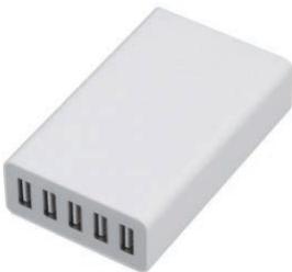
Model: K-MU014 Input: AC 100-240V/50-60Hz Output: USB*5 5V 2.4A each Port, Total 25W; Dimension: 98*60*26mm Weight: 155g
