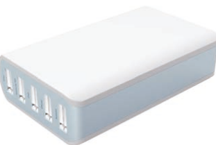
Model: K-MU012 Input: AC 100-240V/50-60Hz Output: USB*5 5V 2.4A each Port, Total 25W; Dimension: 98*60*26mm Weight: 155g
