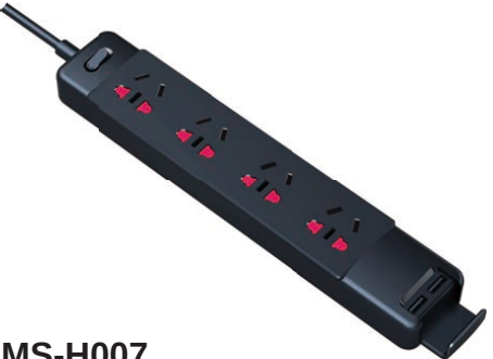
MS-H007 Power: 2500W Input: AC 100-240V 50-60Hz Output: 250V/10A single USB 5V/2.4A 2*USB 5V/2.4A Dimension: 263*50*27mm
