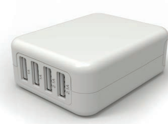
Model: K-MU10 Input: AC 100-240V/50-60Hz Output: USB*4 5V/2.4A each Port, Total 24W; Dimension: 72*55*26mm Weight: 108g
