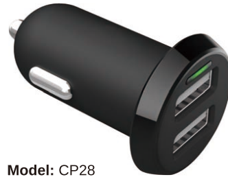
Model: CP28 Input: DC 12-24V Output: USB*2 5V 2.4A each port, Total 5V/3.4A Plastic Housing, LED Light Power indicator Dimension: 50.5*29.8*20.6mm Weight: 20g
