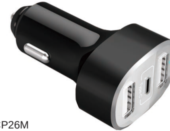
Model: CP26M Input: DC 12-24V Output: Type C 5V 3A USB-A1/2 5V 2.4A each port, Total 24W Aluminum + Plastic housing Dimension: 67*39.5*26.4mm Weight: 35g
