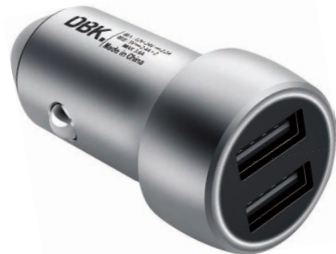
Model: CC140 Input: DC 12-24V Output: USB*2 5V 2.4A each port, Total 5V/3.4A Chromed Copper, Blue LED light in circle Dimension: 73.4*25.4*20.3mm Weight: 45g
