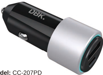
Model: CC-207PD Input: DC 12-24V Output: Type C PD3.0 5V/3A, 9V/2A, 12V/1.5A USBA 5V/3A, 9V/2A, 12V/1.5A Total 18W Aluminum +Plastic housing, LED light Dimension: 59*25.4*23.6mm Weight: 21.5g
